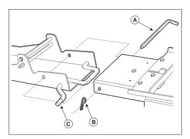
Figure 12. Attaching Snow Blade to Hitch
